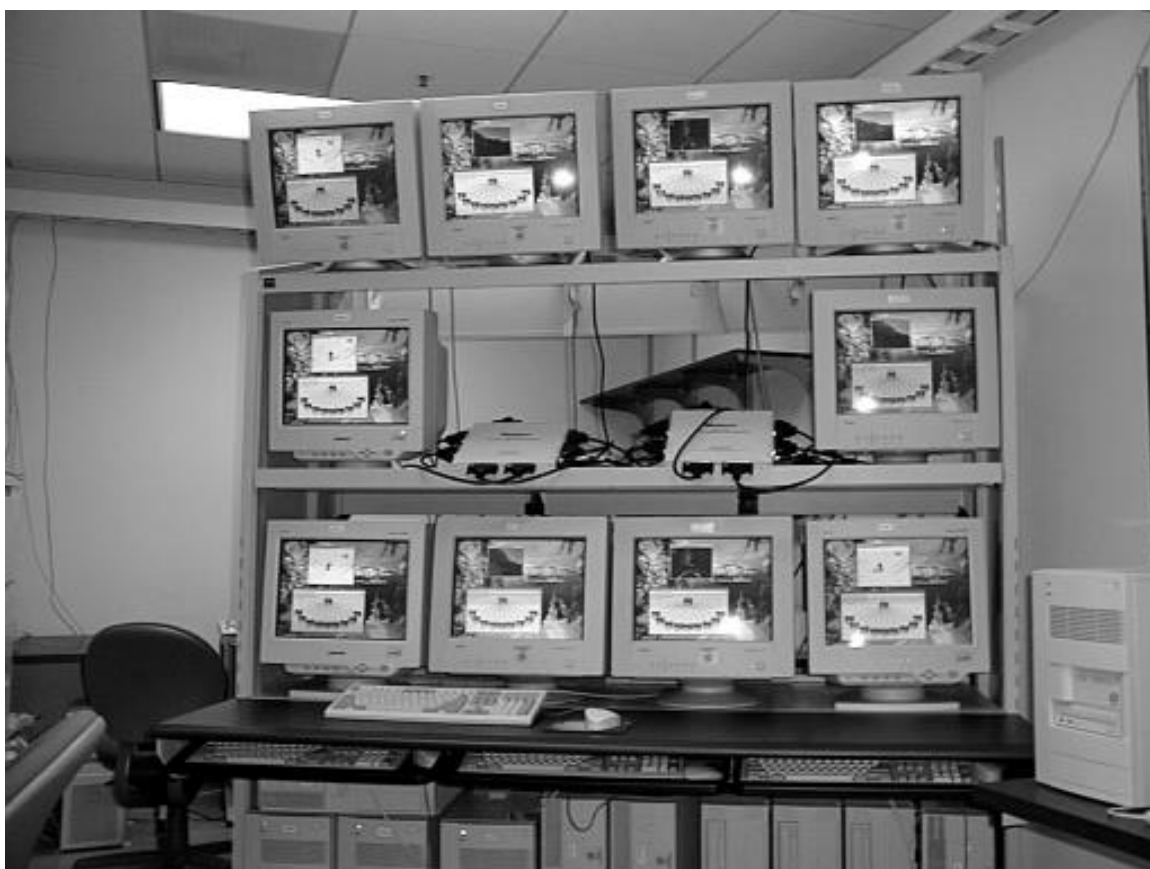
Figure 14: The RAIN System. This is a ten node system. There are ten computers down below, ten screens up on the rack, and Myrinet network switches in the center. They are running a video demo as well as the basic system monitoring software.
