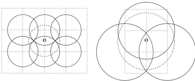
Fig. 2. **Scaling the picture.** On the left hand side of the figure, the dashed line disc requires six discs centered at lattice vertices to be fully covered. On the right hand side of the figure, it requires only three discs.
